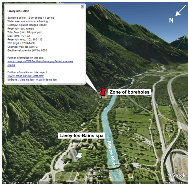
Figure 3: Example of Lavey-les-Bains geothermal site implemented in the Google Earth free software. Visualization of general information about this site is possible while clicking only once on the red pinpoint. Two Internet links allow returning to the homepage of BDFGeotherm in the CREGE website.
